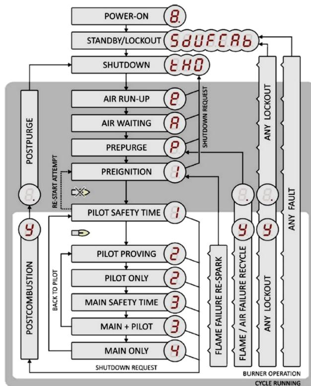
A self-test is performed at power supply-on. Once successfully completed burner is ready to start and use.
