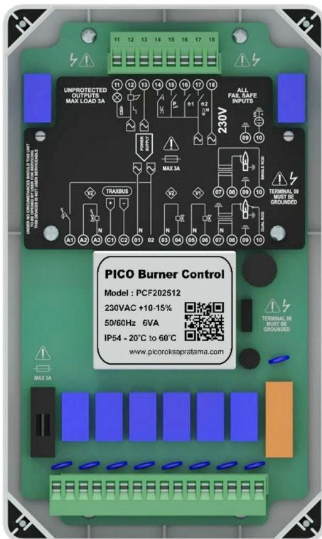
MAKE JUMPER A1-A2 WHEN THE AIR PRESSURE SWITCH IS NOT INSTALLED AND AIR OUTPUT VA PARAMETER IS ENABLE.
