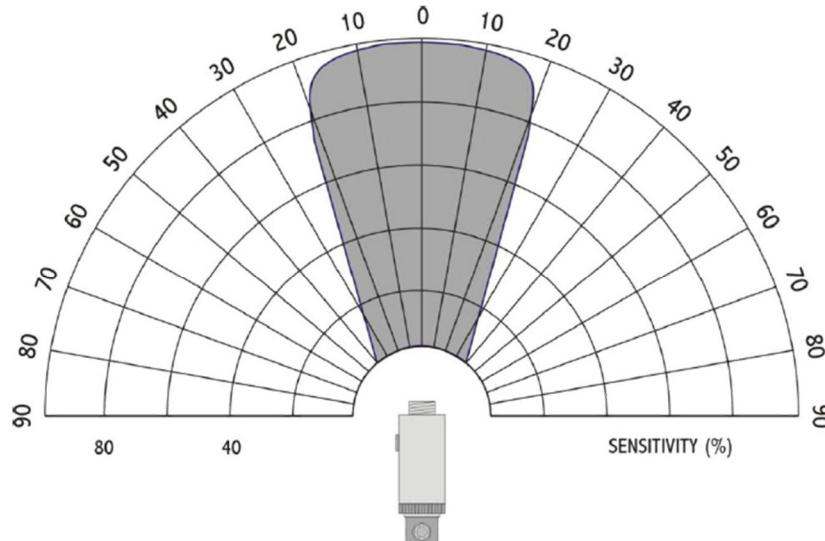
This sensor features a high temperature and high sensitivity ultraviolet (UV) tube, checks a short-circuited or runaway for monitoring gas or oil flames which cycle on and off frequently.
